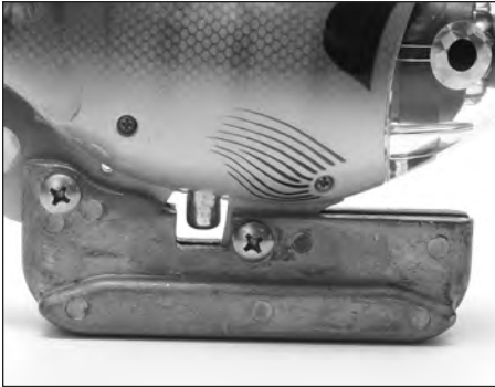
Attach Ballast Weights using included Hardware
